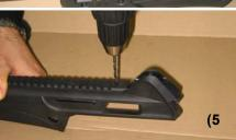
The top rail will now act as a template to drill through the thin polymer membrane that covers the rear two holes. Using the 4mm (or 5/32") drill bit, gently drill through the material in the rearward hole (closest to the rear sight). If using an electric drill or driver, be careful - there is very little material and you will drill through it very easily. See Photograph 5.
